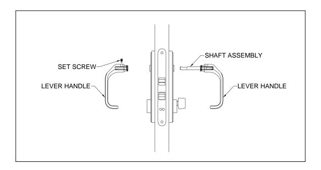
4. Now remove the two screws that are attaching the lockcase and slide the entire lock case out of the door.
