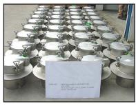
Inspection ports for floating pontoons, aluminum covers and galvanized steel coamings.
