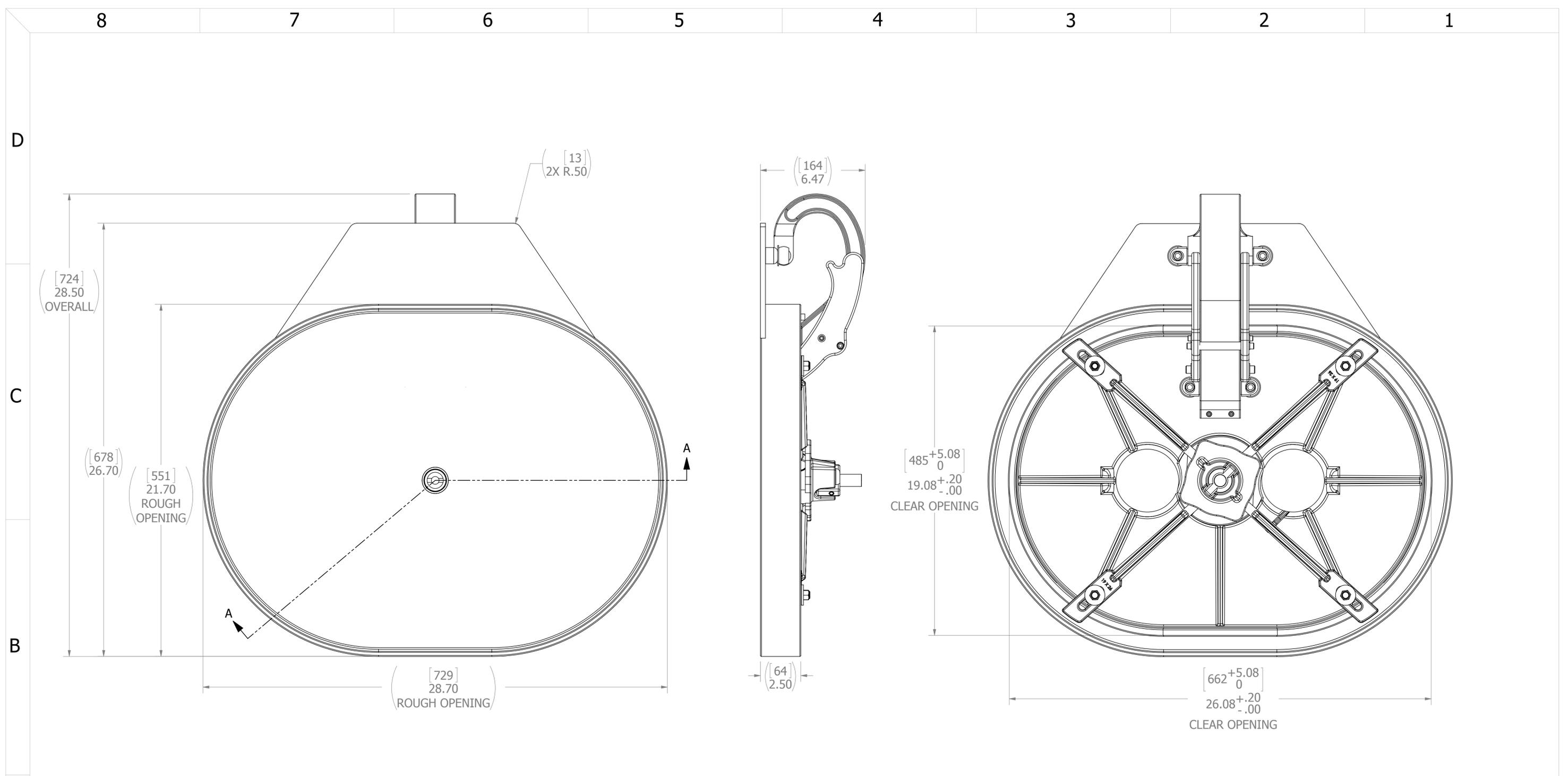
8. THIS DRAWING PROVIDES THE GENERAL CONFIGURATION OF A HATCH. FOR SPECIFIC INFORMATION CONTACT ADVANCED MARINE TECHNOLOGIES SALES.
